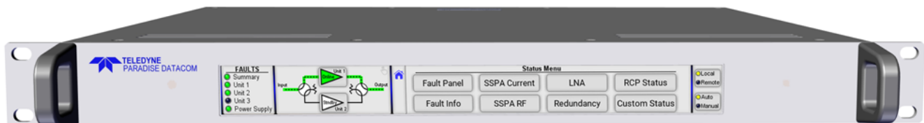
Redundant System Controller Configured for 1:1 Redundant Mode
