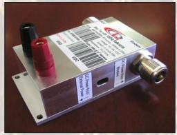
This small and efficient unit provides 10MHz high stability (10<sup>-8</sup>) reference and DC supply to a BUC in case a modem neither cannot supply sufficient power nor 10MHz reference. The unit passes L-Band signal and injects 10MHz reference signal or up to 6A DC current.
