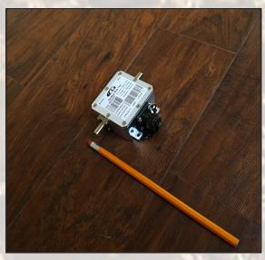
This small and efficient unit provide DC supply to a BUC (DC power supply separate) in case a modem cannot supply sufficient power or doesn't provide BUC power at all. The unit passes L-Band signal and 10MHz reference signal and inject up to 6A DC current.
