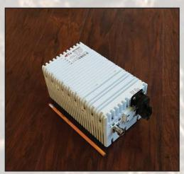
This smallest and lightest 100W L-To C-Band Block Up Converter is based on GaN technology. It is designed to be mounted on the feed horn. The unit covers C-Band sub-band Insat (6.725-7.025 GHz)
