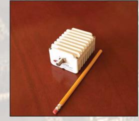
This smallest and lightest 5W L-To Ku-Band Block Up Converter is based on GaN technology and is designed to be mounted directly on the feed horn. High power efficiency resulting in low current (< 1 amps) consumption allows to use this BUC with any modem without an external power supply.
