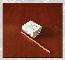
This smallest and lightest 2W L-To Ku-Band Block Up Converter is based on GaAs technology and is designed to be mounted directly on the feed horn. High power efficiency resulting in low current (<1 amps) consumption allows user to pass DC supply voltage via IF cable. The unit is ideal for network and point to point, data distribution, portable and emergency applications.
